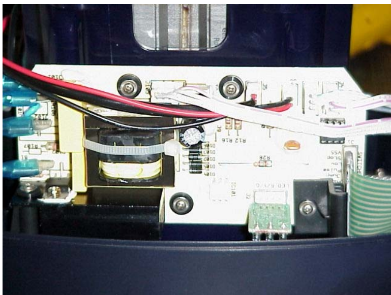
Figure 2. PC Board. Shown without Mylar Shield.
