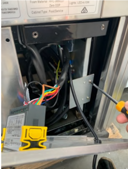
Remove screws and slide panel out for easier access
