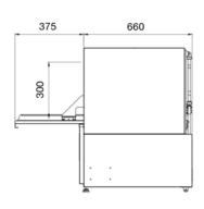
The Cafemate Advanced Wash Control model is a compact underbench dishwasher with a usable height capable of taking care of 30cm plates. Installation and superior cleaning is made easy with its standard pump out drain and detergent/rinse aid injectors.
